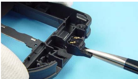
Use tweezers to remove the microphone.
