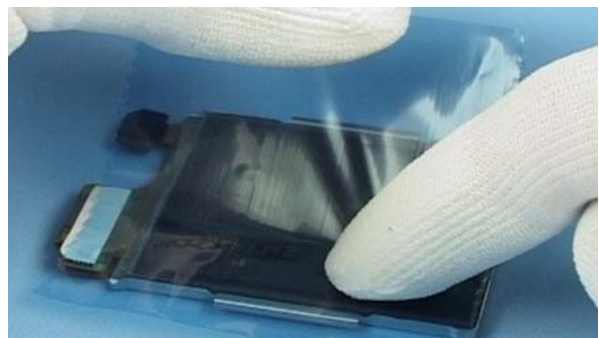
Protect the LCD module with a film.
