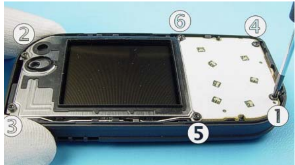
Unscrew the six Torx Plus® size 6 screws. For assembly, the reverse order and a Torx Plus® driver with a torque of 22Ncm has to be used.
