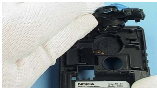
Turn the B-cover as shown in the picture and remove the IHF lid.
